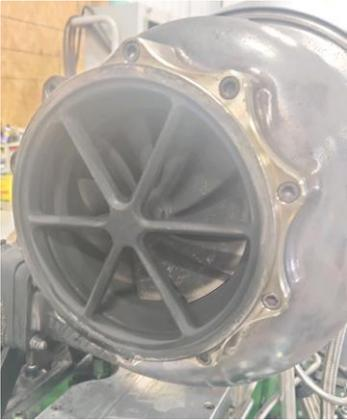
B) -Exhaust housing has the capacity of installing 2 – ½ inch bolts installed 90 degrees of each other. Welded or fastened.
