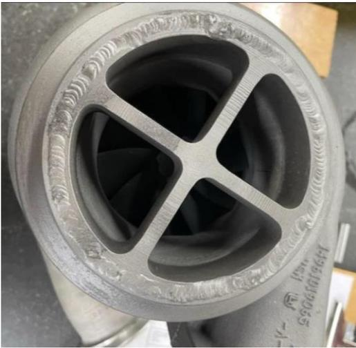
E)- Exhaust adapter must be fabricated using two interlocking pieces of .250-inch x 1.000-inch flat steel notched .250-inch x .500-inch at center creating a single interlocking assembly and welded into a cross pattern.
