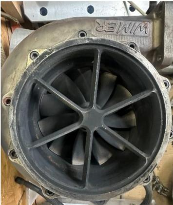
B) -Exhaust housing has the capacity of installing 2 – ½ inch bolts installed 90 degrees of each other. Welded or fastened.
